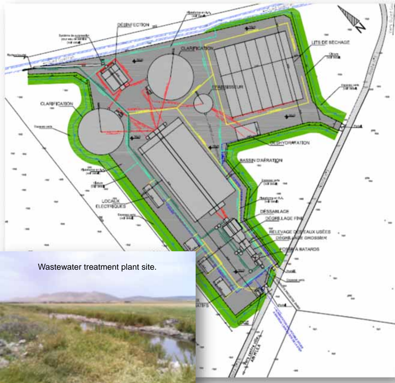
Wastewater treatment plant general layout.
